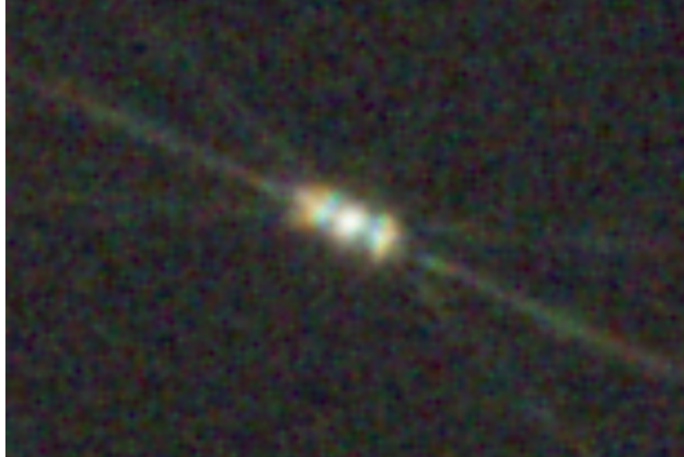
Figure 3, Diffraction Spikes from Bahtinov Mask
